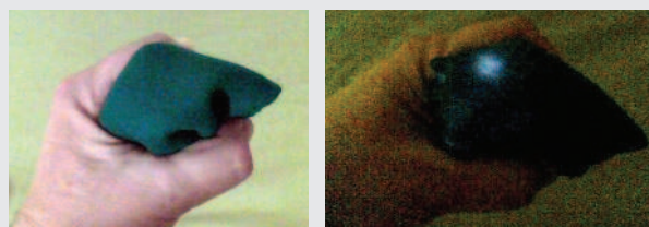
Fig. 19a and 19b: Felt completely blocks visible light but not infrared.
