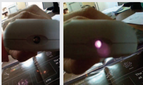
Fig. 17a: Remote activated naked eye. Fig. 17 b: Remote activated by mobile phone.
