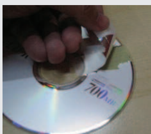
Fig. 10b: Removing the metal layer of the CD, with tape.
