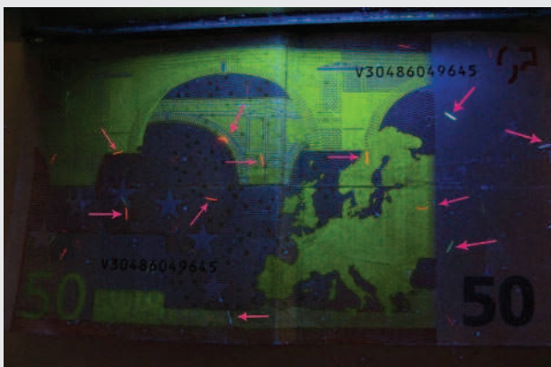
Fig. 26: A note of 50 illuminated with UV light, shows small fluorescent strips marked here by arrows.
